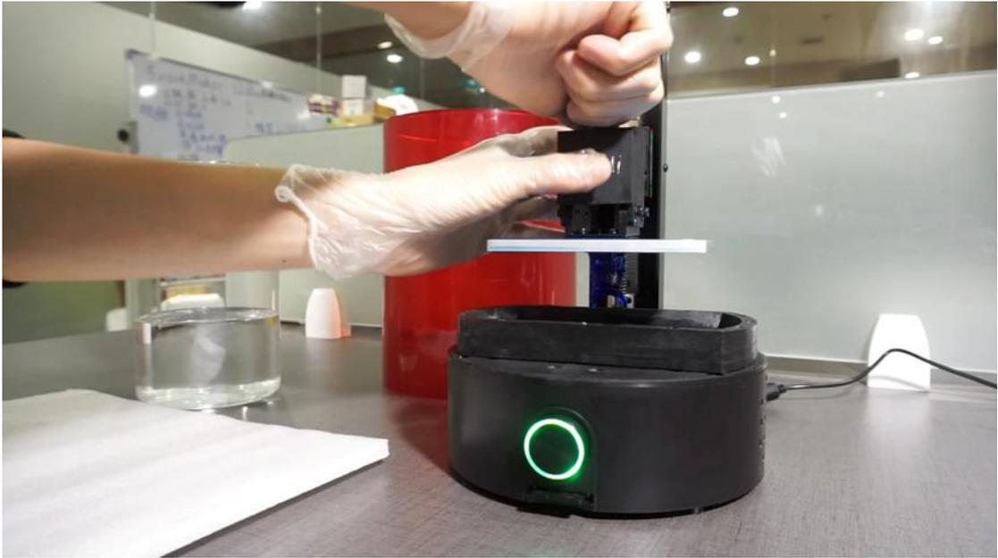
Step11: Loosen the handle and remove the platform.
