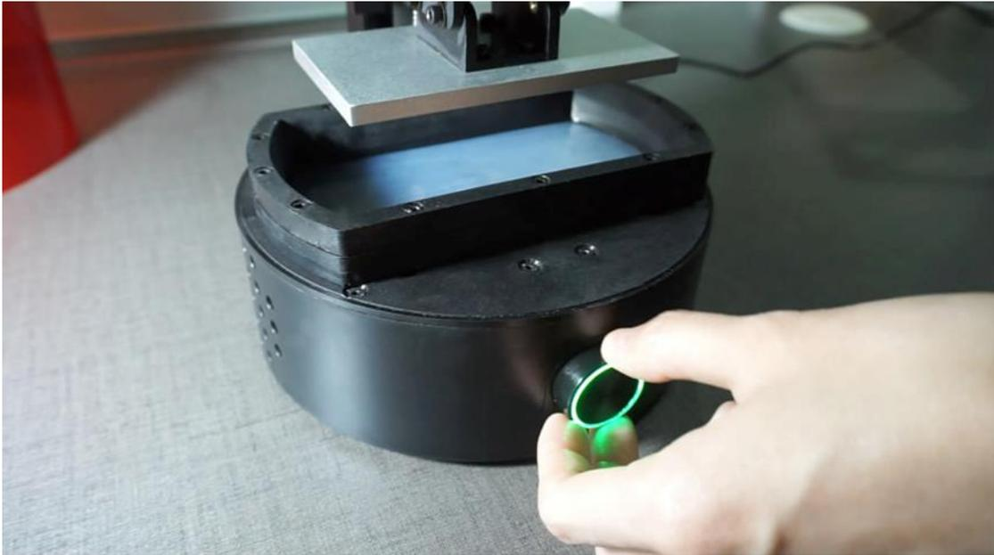
Step5: Rotate the knob drops the platform to the lowest point.
