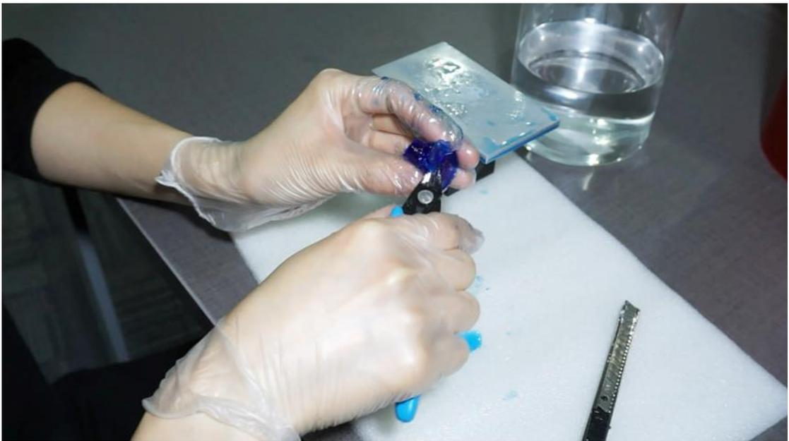
Step12: Remove the supports of model.
